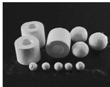
Fig. 12. Some examples of molded binderless zeolites.
