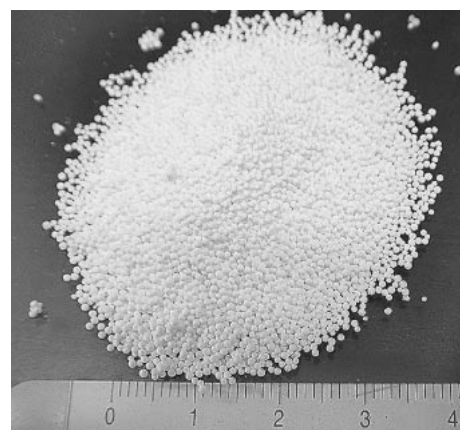
Fig. 16. An example of a molded binderless zeolite (ZSM-5).
